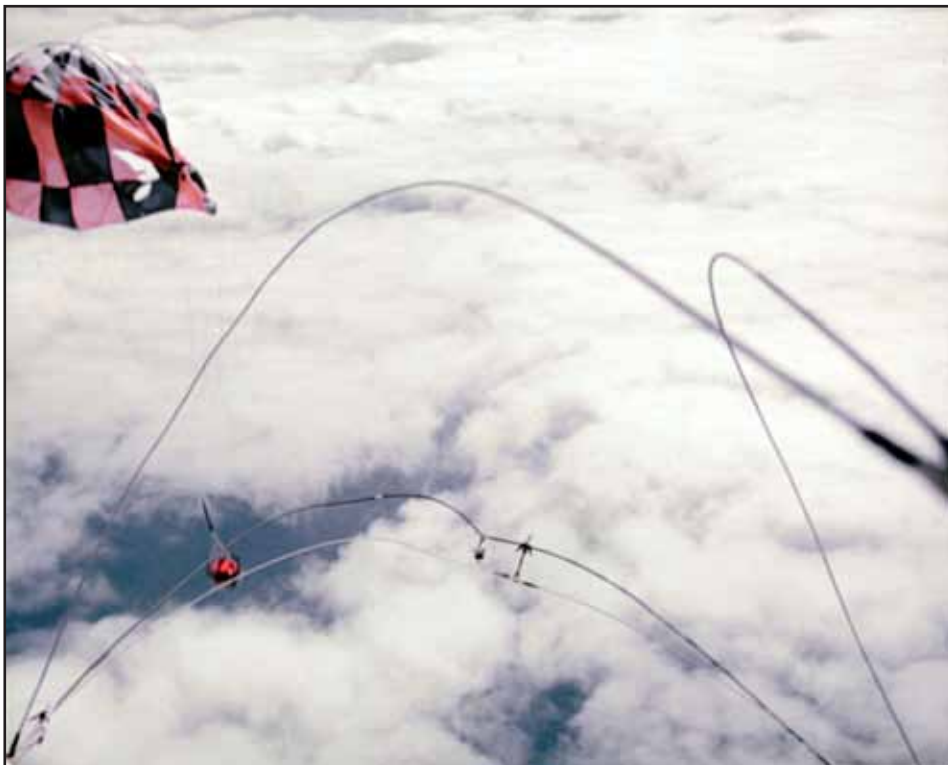
The Discoverer 17 parachute and capsule on November 14, 1960. The loop is deployed and in trail. In this photo it appears that the chute has been hit and torn by the right pole, but the hooks remained taped to the poles./Photo credit: USAF
