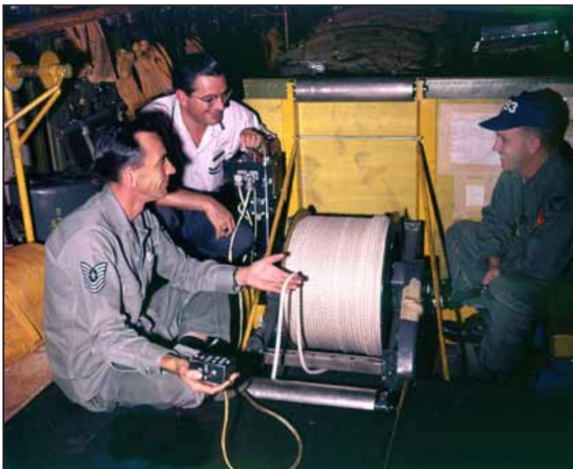
MSgt Willie Stanberry, winch operator and recovery section Noncommissioned Officer in Charge (NCOIC), holds a piece of winch rope and the winch control box, while TSgt James Cross and All American Engineering technical representative Harry Conway look on. The winch control box was on a long electrical cord so the winch operator could move around the recovery deck with it. Behind MSgt Stanberry's head is a rear pole support. The large box-like structure behind the men covers the two 500-gallon Benson fuel tanks./Photo credit: USAF
