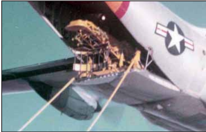
JC-130B dolly in the raised position with the capsule cradle tilted outward—poles down and unriggered. In this photo the fairlead is down and the capsule cradle or carriage is tilted outward. This is the configuration of the rig when a heavy package has been reeled up to the fairlead and is about to be set into the capsule cradle, Edwards AFB on April 17, 1961./Photo credit: USAF
