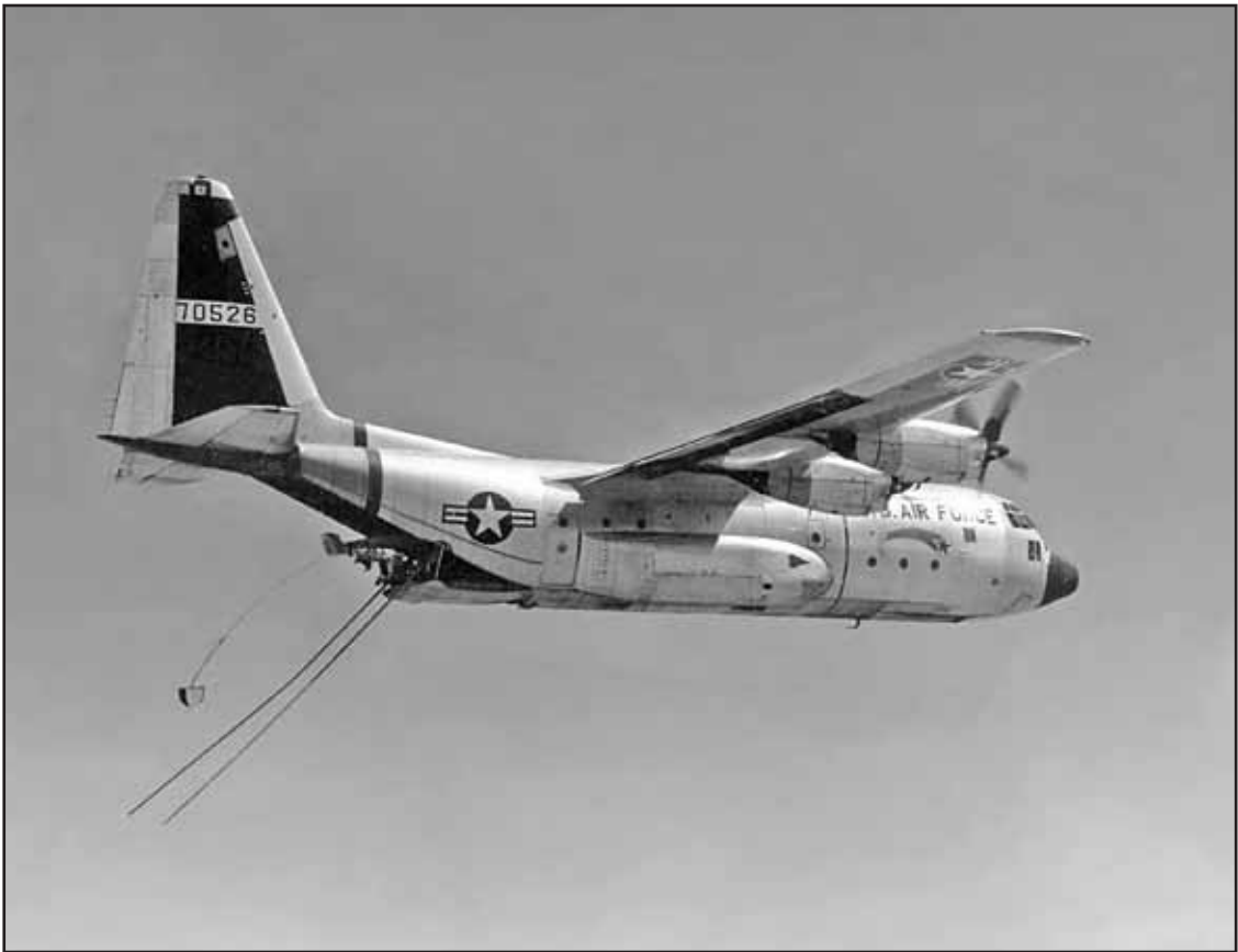
JC-130 reeling in a test capsule at Edwards AFB in 1961./Photo credit: USAF
