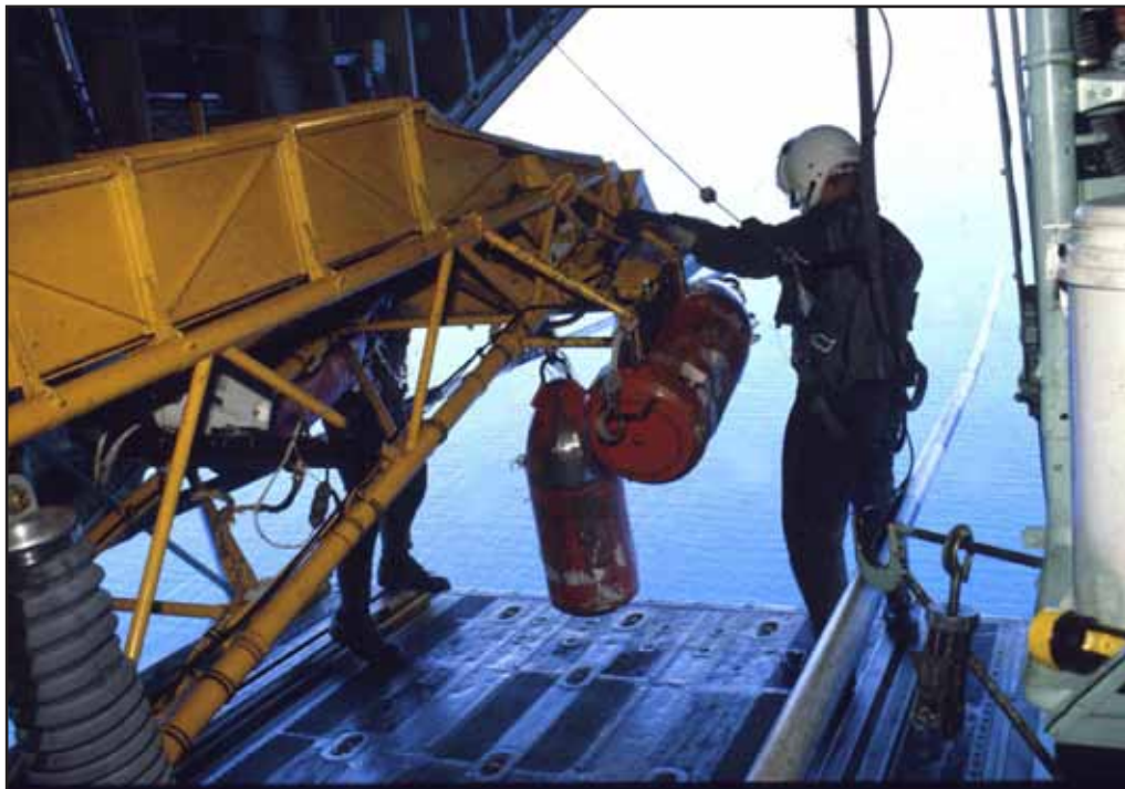
An aft JC-130 loadmaster standing between the dolly to his left and the extended recovery pole to his right. The red training payload dangling at the left has just been recovered and reeled up to the fairlead of the dolly. /Photo credit: USAF
