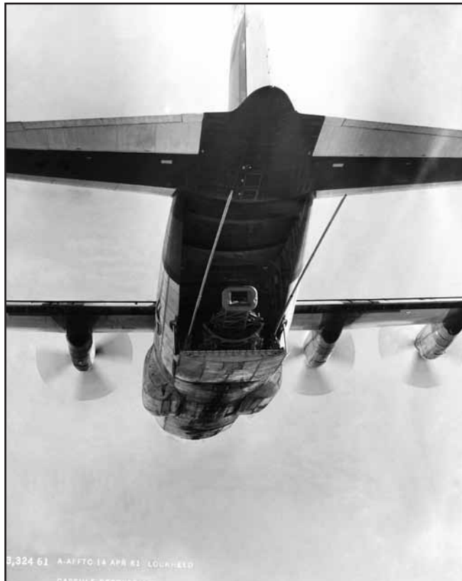
JC-130 in 1961 with its dolly in the rear position on the ramp and the recovery poles without a loop. This is most likely at Edwards AFB photographing the aircraft and recovery equipment, not a recovery. /Photo credit: USAF
