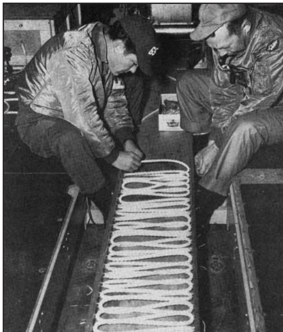
Left: A C-119J winch and trough with the zigzagged recovery rope in 1958. Right: Loadmasters A1C Billy Gurganious (left) and A1C Walter Johnson tying a recovery rope inside a C-119J trough. /Photo credit: USAF
