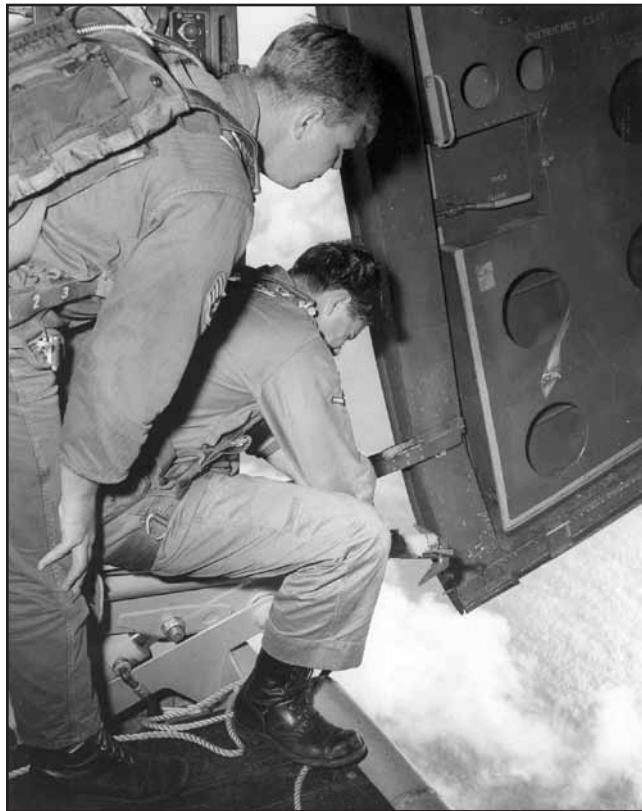
A C-119 loadmaster taping a recovery hook to a pole./Photo credit: USAF
