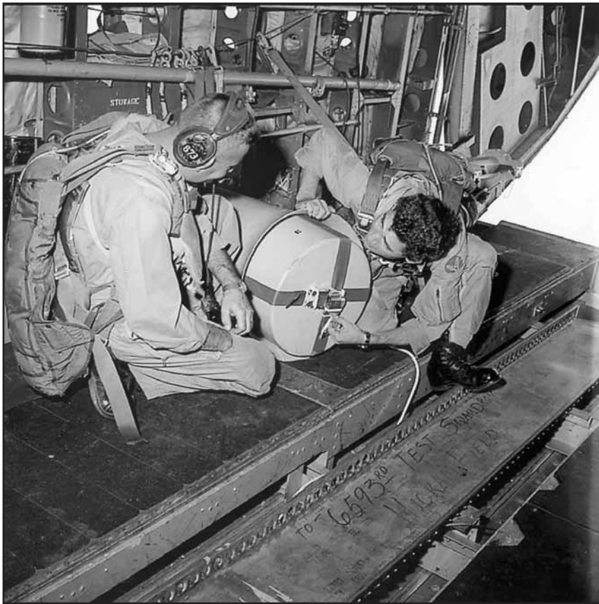
Crew members prepare to remove the canister from a recovered data capsule. The person on the right has his foot on the edge of the trough. Each one of those little holes in the trough had a pin on the other side of it to which we had to tie one of the bends in our accordion folded rope. Lots of ties! And we had to retie each time we rigged for another recovery./Photo credit: USAF
