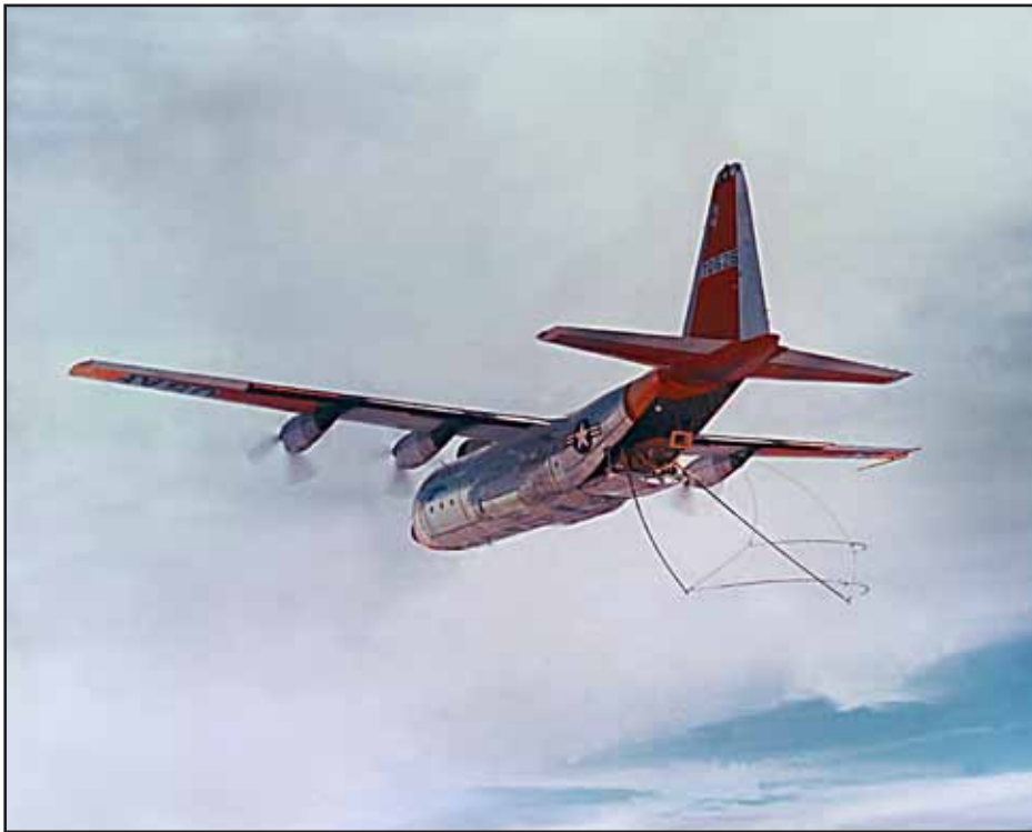
JC-130B during a parachute recovery flight test at Edwards AFB, circa 1960./Photo credit: USAF
