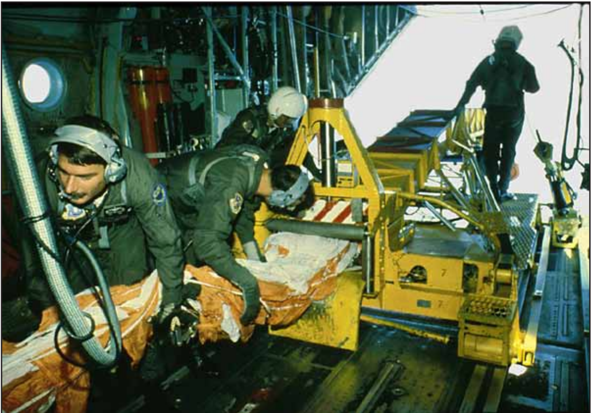
The recovery crew handles a recovered chute as it is winched in through the trough toward the winch./Photo credit: USAF
