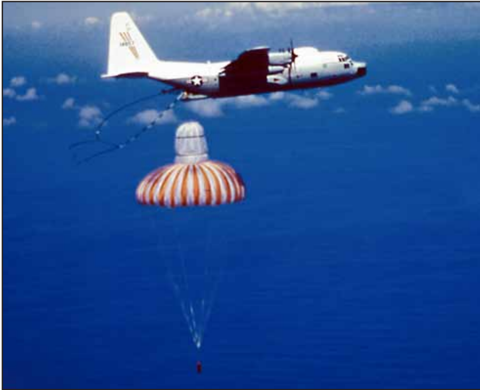
JC-130 about to recover the white cone (or conical extension) of a Mark 8 parachute. The cone had reinforcement lines that were snagged by the JC-130 hooks during a recovery./Photo credit: USAF
