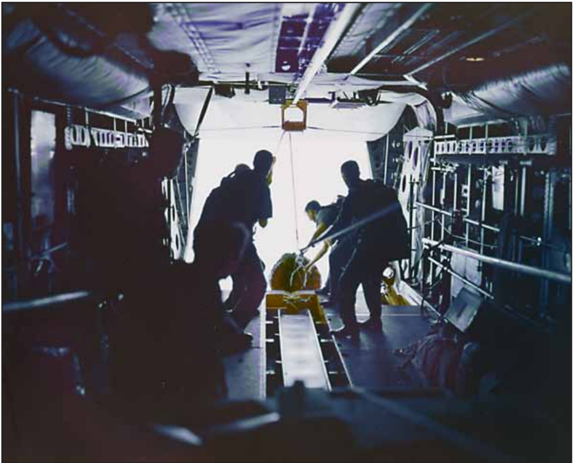
Crew hoisting a capsule into the aircraft in 1959. The crew is using the overhead sheave roller to pull the capsule upward and over the back of the deck./Photo credit: USAF
