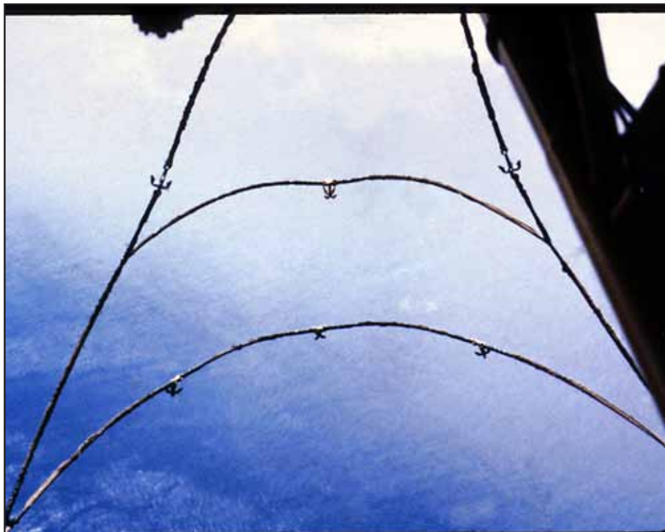
A parachute recovery rig (poles, line, and hooks) suspended below the rear of a JC-130 preparing to recover a parachute./Photo credit: USAF
