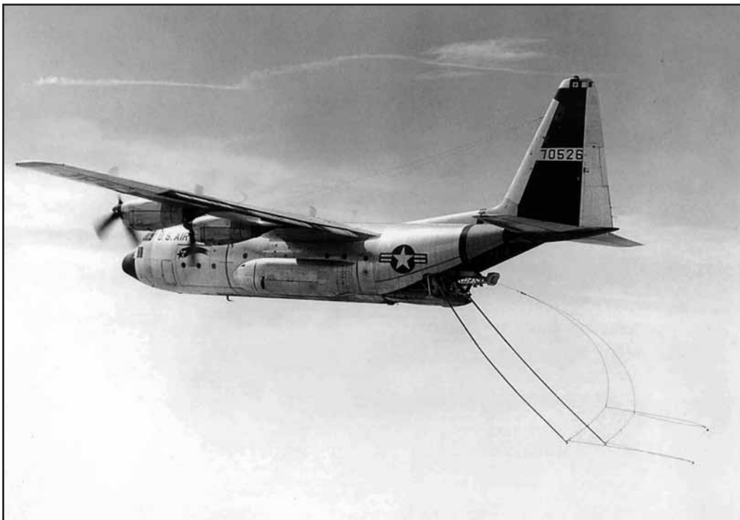
JC-130B #70526 with poles down and loop in trail at Edwards AFB on April 17, 1961./Photo credit: USAF
