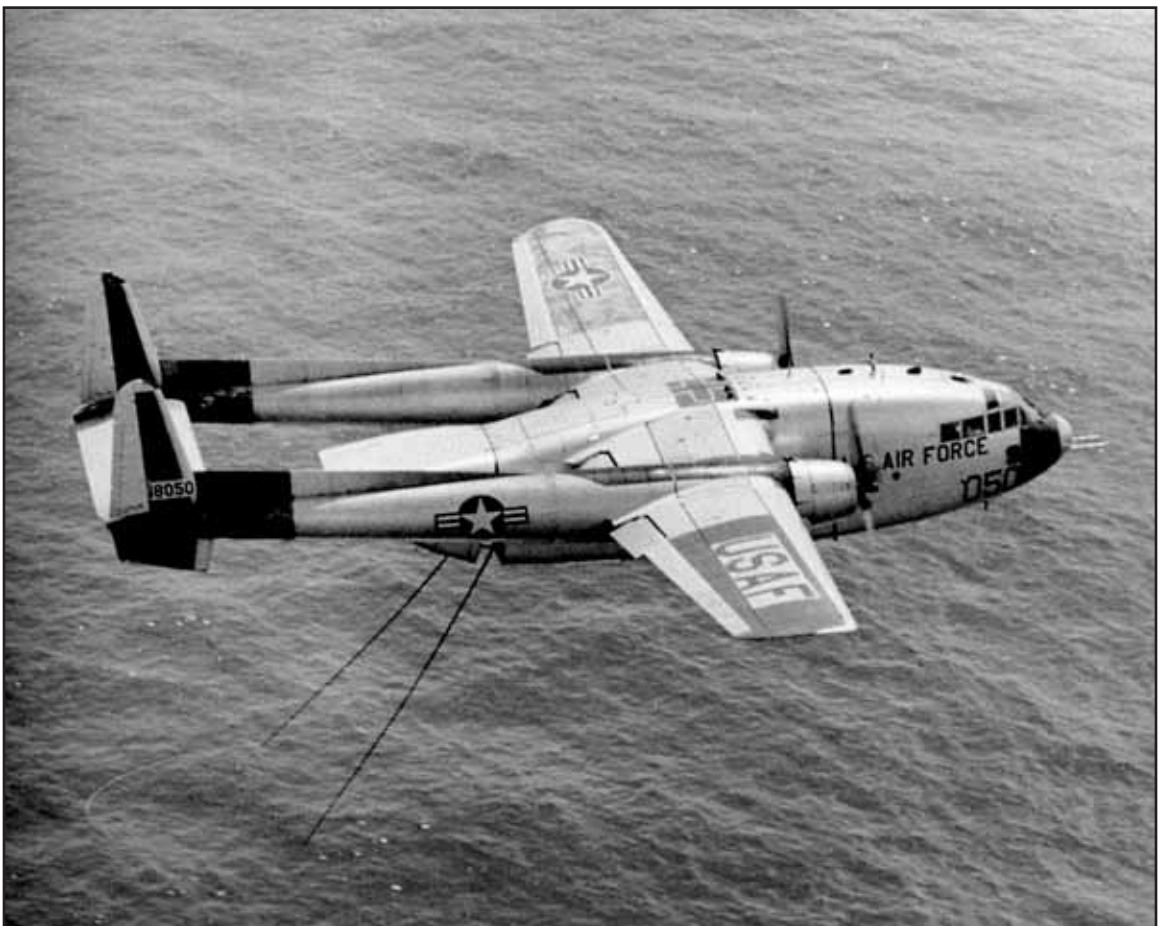
C-119J about to recover a floating training capsule in 1960./Photo credit: USAF
