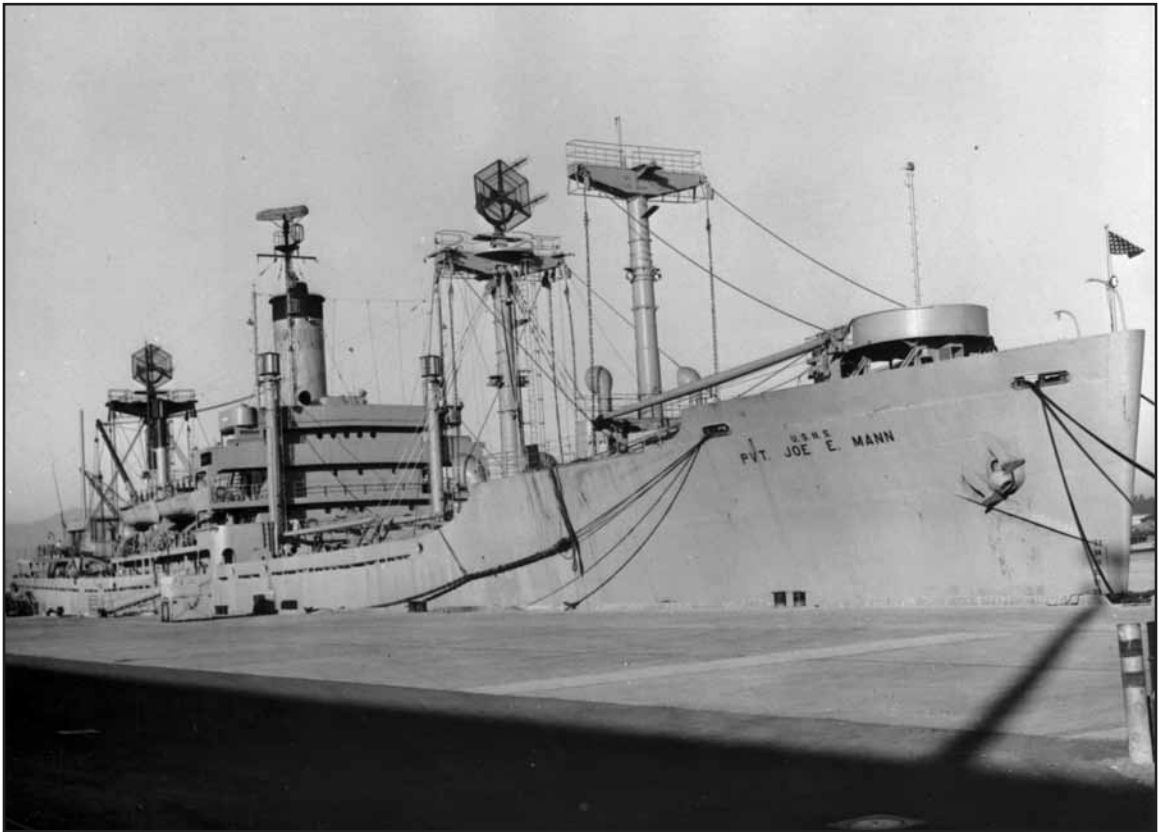
An instrumentation ship (USNS PVT Joe E. Mann ) in 1960 that supported the Discoverer program. The ship was positioned between the tracking stations at Kaena Point, Hawaii and Kodiak, Alaska and received telemetry from the Agena and the reentry vehicle during a Discoverer mission./Photo credit: USAF
