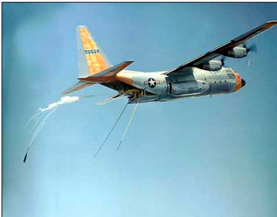
JC-130 recovering a test package and parachute in 1962. The package is probably an expended jet-assisted takeoff (JATO) bottle filled with shot. JATO bottles were often used during flight test recoveries at Edwards AFB./Photo credit: USAF
