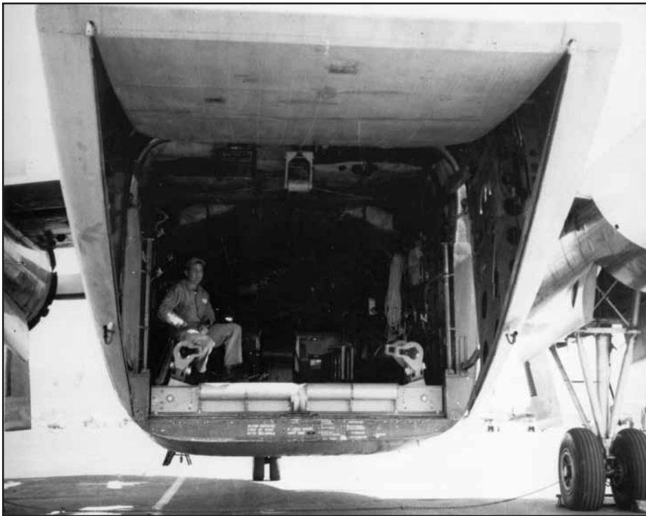
A beavertail door on a C-119 that could be opened upward while in flight to recover parachutes. /Photo credit: USAF
