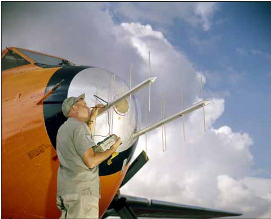
A noncommissioned officer inspecting the homing antennas on a C-119J of the 6593d at Hickam AFB in 1960./Photo credit: USAF
