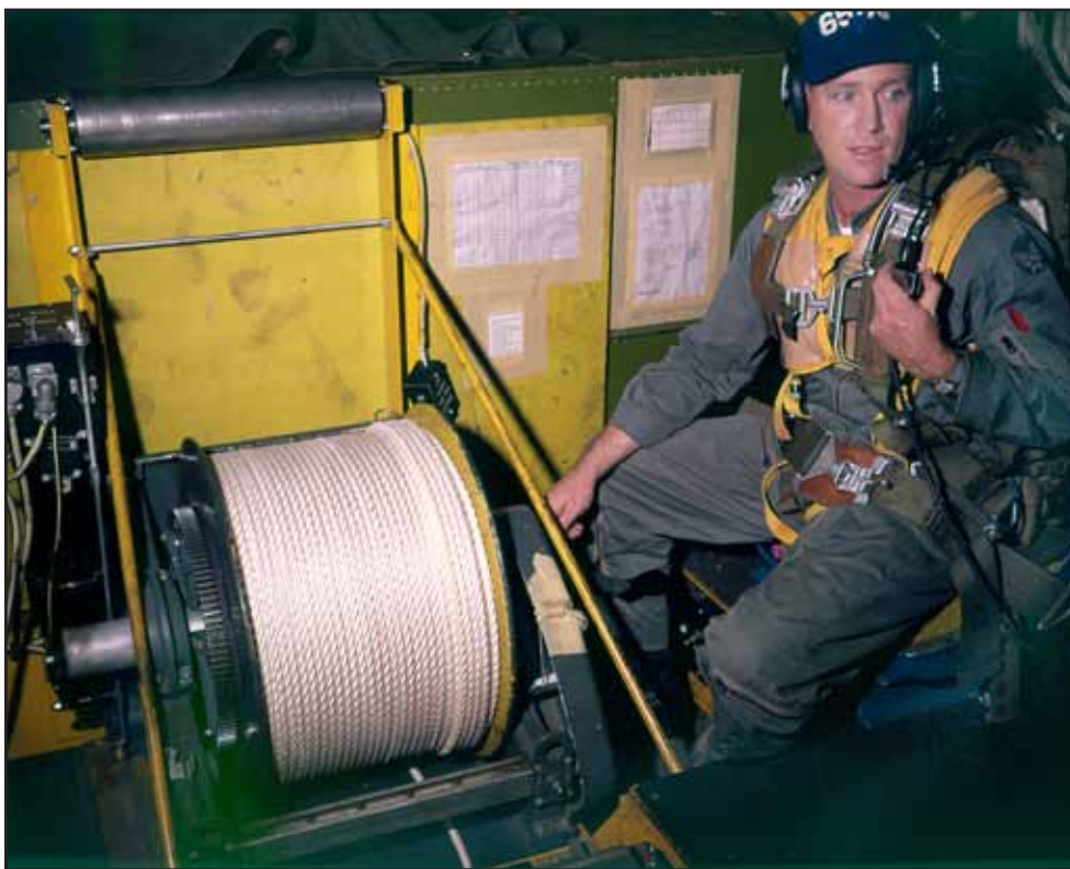
C-119J winch operator TSgt James Cross of the 6593d beside his parachute recovery winch wound with nylon recovery rope in 1960./Photo credit: USAF
