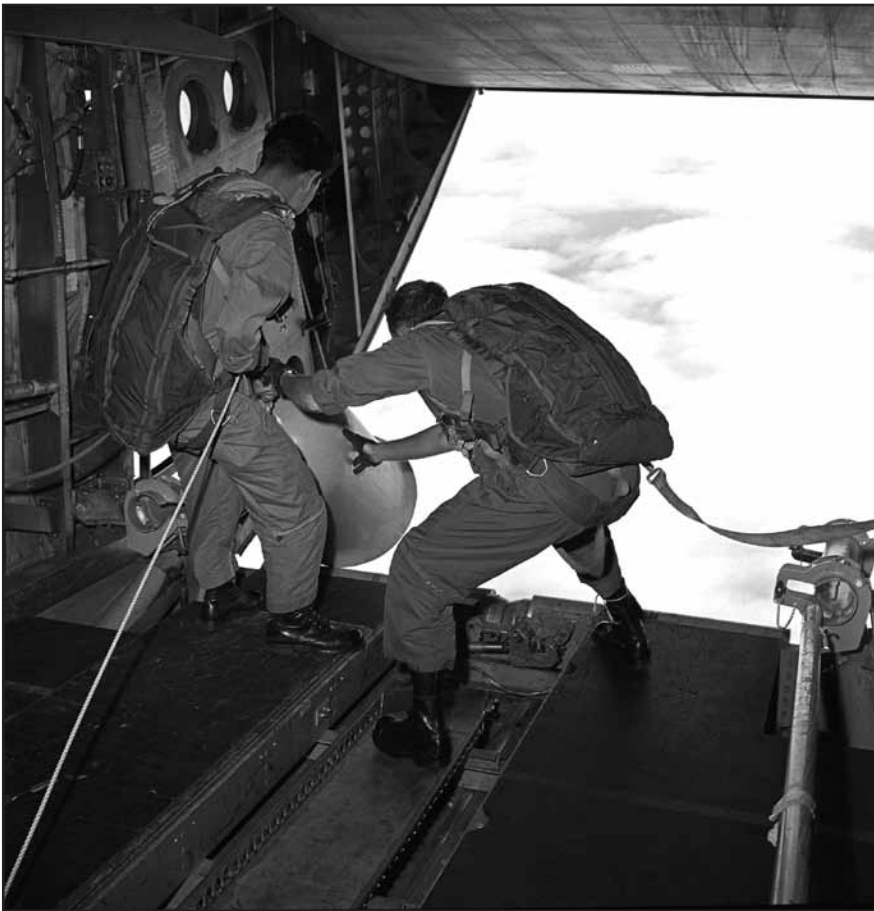
Two C-119J loadmasters hauling in a data capsule recovered from a ship in 1960./Photo credit: USAF
