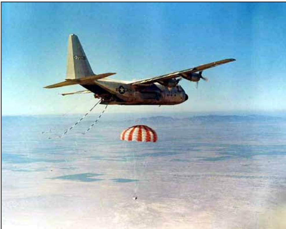
JC-130 recovering a parachute and payload in 1961 at Edwards AFB./Photo credit: USAF
