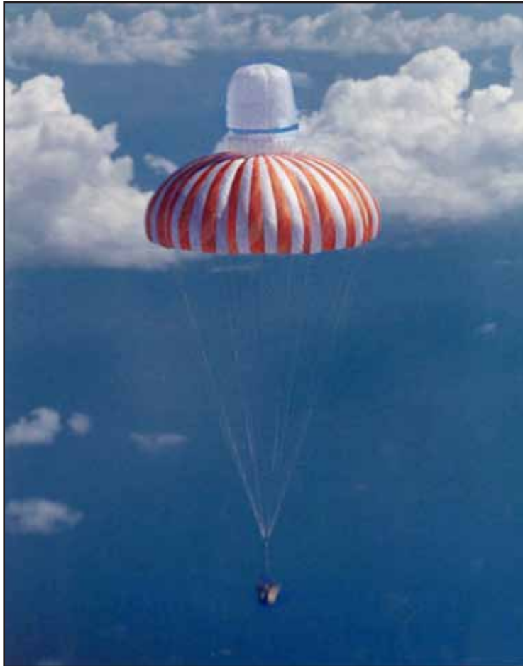
Mark 8 parachute with an unknown payload. The JC-130 would strike the small white parachute with its recovery gear when recovering these parachutes. /Photo credit: USAF
