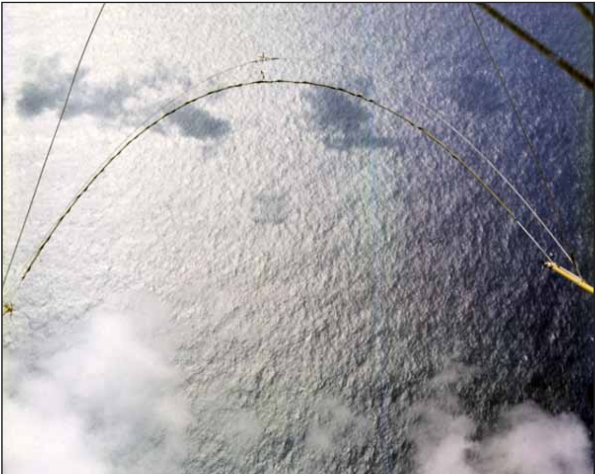
Recovery lines and hooks trailing below a C-119J during a 1959 training recovery./Photo credit: USAF
