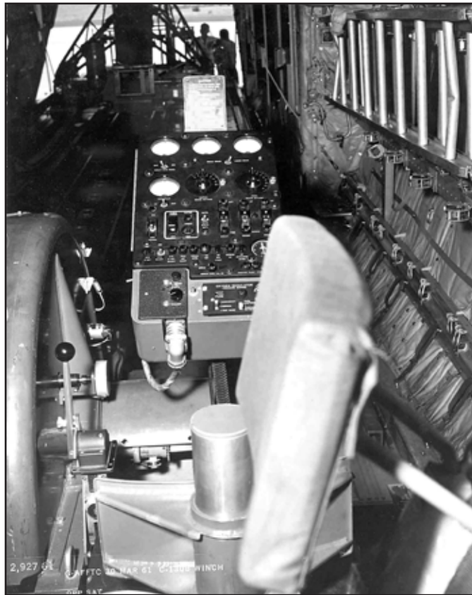
Looking back from winch operator's position, March 1961. The photo shows the winch operator's console, part of the winch and the dolly at the back of the aircraft./Photo credit: USAF
